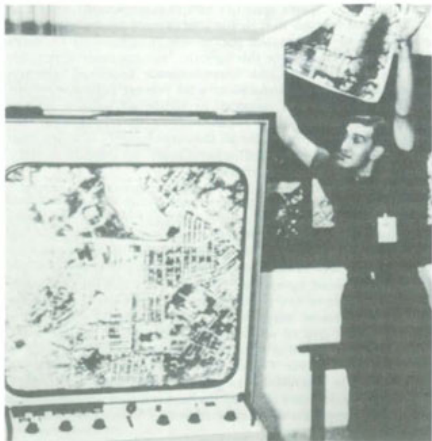
IMAGERY INTERPRETER removes photocopy produced by the Itek variable-width viewer with printer.
